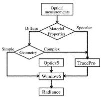
Figure 1. Process flowchart showing the software tools used to arrive at a photorealistic simulation of an interior space.
