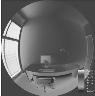
Figure 2b. Falsecolour luminance map (cd/nf) rendered without use of BSDF data. Matte-VB: January 15, 10:00 AM.
