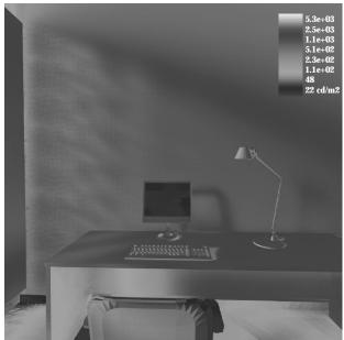
Figure 3a. Falsecolour luminance map (cd/nf) rendered with the BSDF data. Mirror-VB, December 21, at 9:00 AM.
