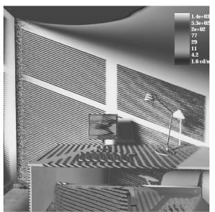
Figure 3c. Difference in luminance (cd/n²) between Figure 3b and Figure 3a (nonBSDF-BSDF).
