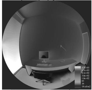
Figure 2a. Falsecolour luminance map (cd/nf) rendered with the use of BSDF data. Matte-VB: January 15, 10:00 AM.
