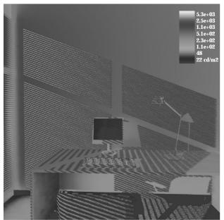
Figure 3b, Falsecolour luminance map (cd/m²) rendered without BSDF data. Mirror-VB, December 21, at 9:00 AM.
