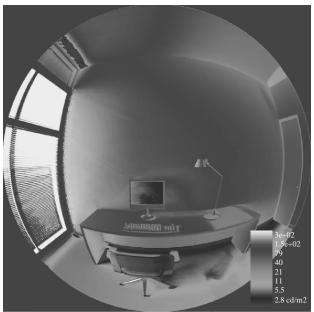
Figure 2c. Difference in luminance (cd/nt) between Figure 2b and Figure 2a (nonBSDF - BSDF).
